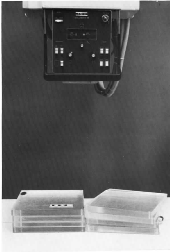
Figure 8.20. Phototimer evaluation test setup. Center the first four sheets under the x-ray tube and directly over the phototimer detectors. Be sure to include date, room, and technique information on each film.
